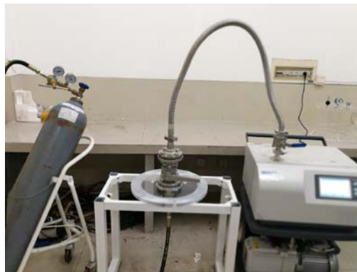
Fig. 7 Leakage detection device for floating ball valve
